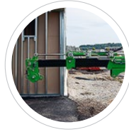
Hydraulic boom extension (800 kg lift capacity)
