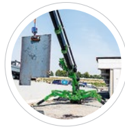
90° rotating magnet 500 kg lift capacity 500 kg
